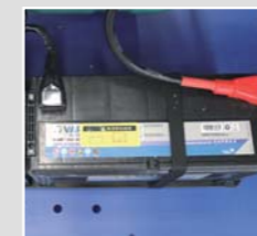
13 High power starter battery installed and connected to the engine, including cables and connectors.
