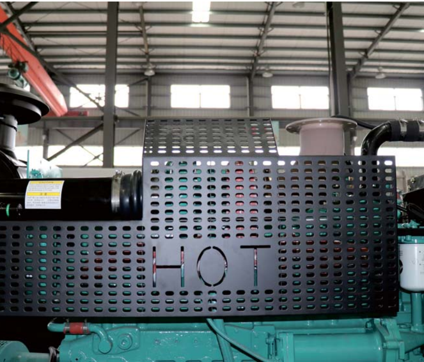
▲ All the hot parts are guarded to avoid accidents caused by touch
