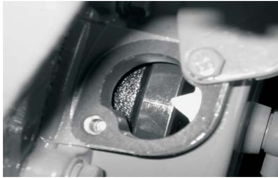
Fig. 3-2 Inspection hole on gear chamber cover
